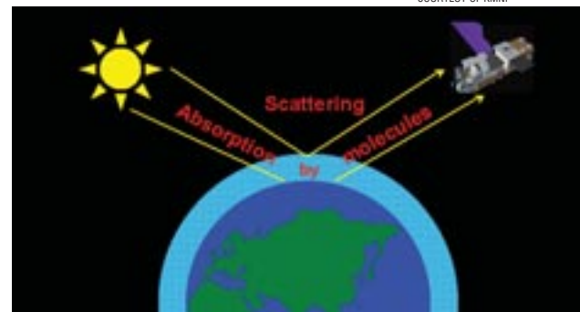
Figure 1. OMI measures UV light that is either reflected from the surface or scattered back from the atmosphere.
