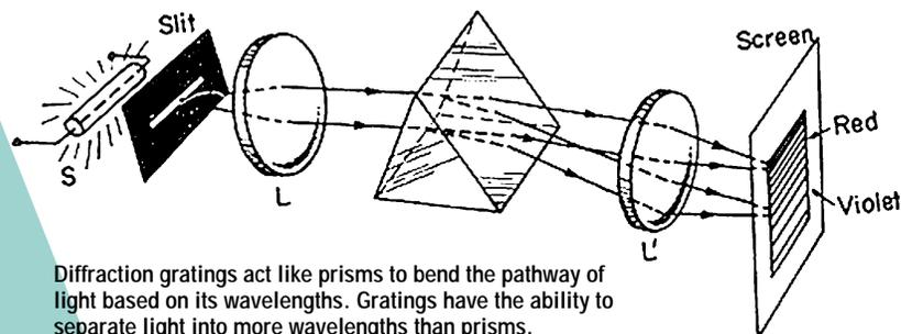
Diffraction gratings act like prisms to bend the pathway of light based on its wavelengths. Gratings have the ability to separate light into more wavelengths than prisms.
