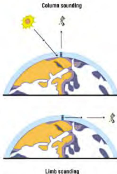
An instrument taking *column soundings* samples the atmosphere from top to bottom, by looking straight down to the surface. An instrument taking *limb soundings*, gathers data from a horizontal slice of the atmosphere by looking out across the atmosphere.
