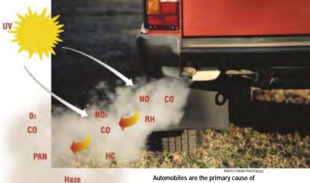
Automobiles are the primary cause of photochemical smog. Every day, exhaust emissions are converted by sunlight to nitrogen dioxide (NO<sub>2</sub>), ozone (O<sub>3</sub>), carbon monoxide (CO), peroxyacetyl nitrate (PAN), and a variety of other pollutants.
