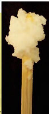
Similar to napalm, when a small amount of the tent waterproofing agent is ignited; it rapidly drips and spreads a sustained fire down a stick.
