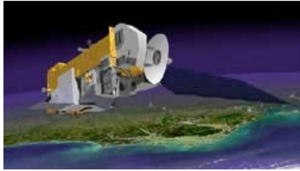
The Aura satellite, seen here in an artist's rendition, houses instruments that monitor the chemical make-up of the atmosphere and help researchers understand ozone chemistry. Credit: NASA
